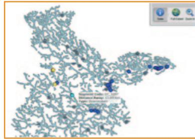
river network, available in Esri's geometric network format. Further processing using custom scripts in the Python programming language permits snapping any point dataset to the river network to create records usable by the River Network Solver.
